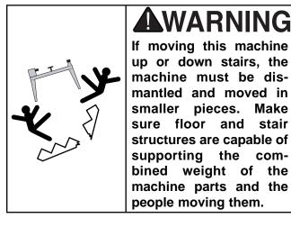
WARNING If moving this machine up or down stairs, the machine must be dismantled and moved in smaller pieces. Make sure floor and stair structures are capable of
